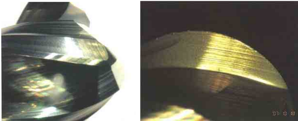
Fig. 5 Left: typical ball end mill with R=2mm and Right: tool cutting edge after cutting.
