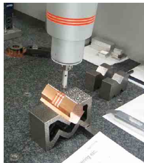
Fig. 8 KEK CMM typical setup.
